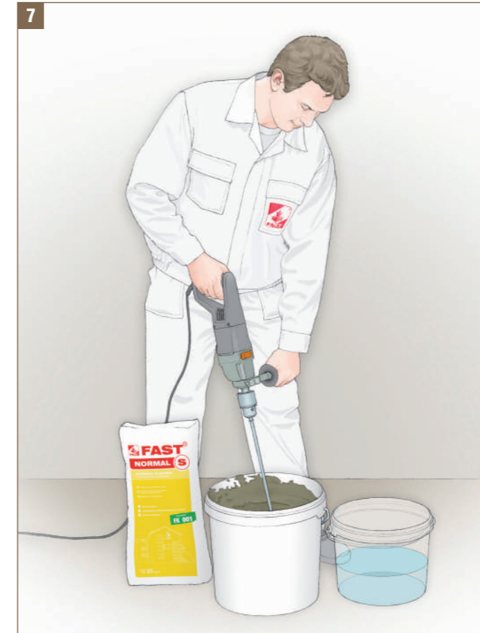
Fig. 7 - Preparation of mortar glue © FAST 2008
