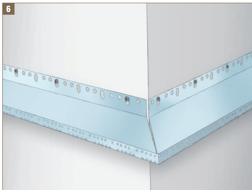
Fig. 6 - Mounting first starter track at the corner of the building © FAST 2008
