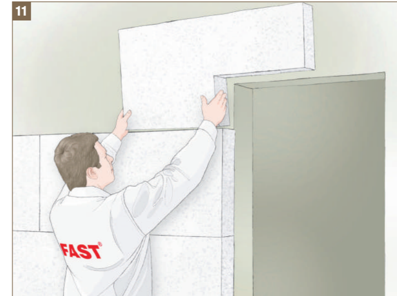
Fig. 11 - Proper arrangement of insulating panels near doors and windows © FAST 2008
